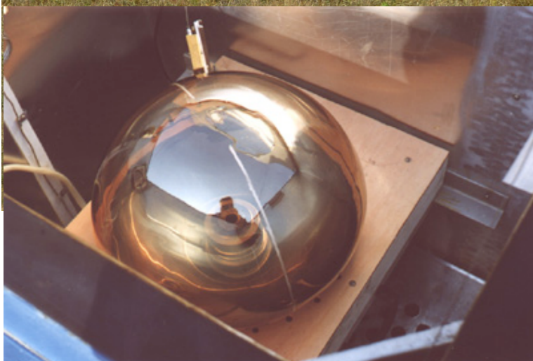
133 non-imaging Cherenkov detectors
