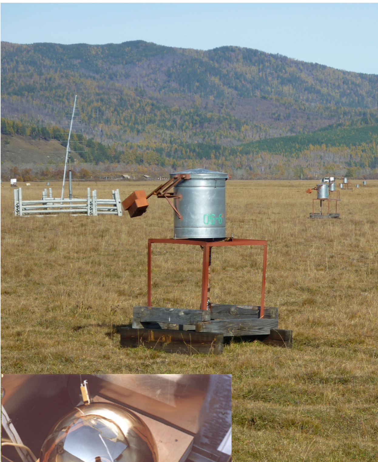
133 non-imaging Cherenkov detectors
